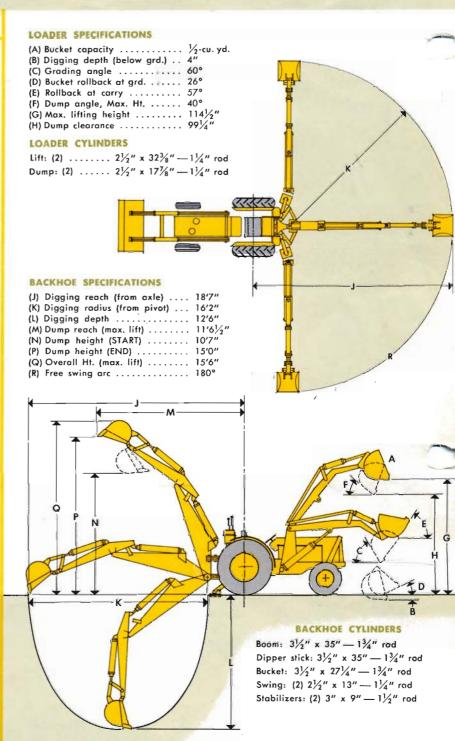
BOOM AND DIPPER STICK: Stress engineered box-welded steel plate construction, reinforced at all strain points. Hardened steel pins and replaceable bushings used throughout. Extra-long dipper stick gives proper angle between boom and dipper stick for maximum digging leverage in all positions.
