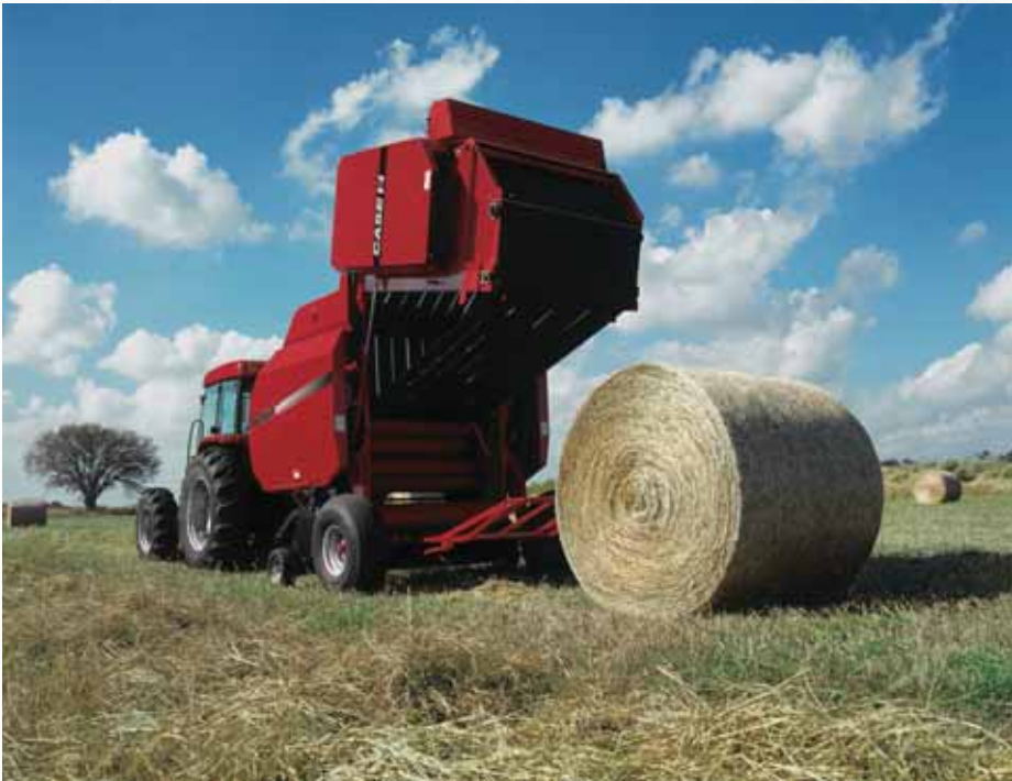
A variable bale chamber on Case IH RB 4 series round balers allows for customizable bale diameter.
