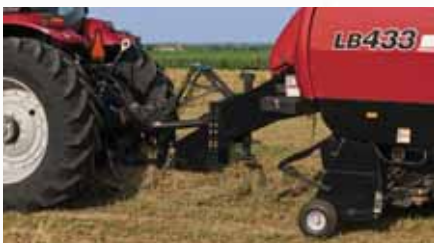
Connecting a LB 3 series large square baler to a tractor is simple with a narrow front frame and hitch
