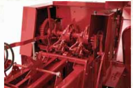
Case IH SB series balers feature dependable gear driven twine knitters
