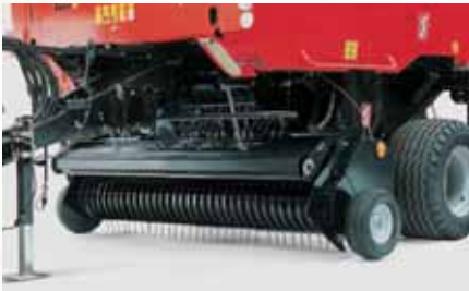
Case IH RB 4 series round baler pickups are substantially wider than the bale chamber.
