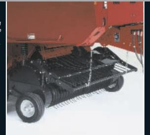
You can adjust the pressure on the bale density system without tools, allowing you to build bales just the way you want them. The easy-to-read gauge on the front of the baler lets you monitor system pressure from your tractor seat. Bale density is controlled hydraulically with a selfcontained system. Requiring little maintenance, this system eliminates problems that can be caused by dirty hydraulic fluid and complicated hydraulic valves.
