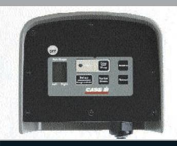
With the Electric-Controlled Twine Wrap System, the bale-shape sensor guides your driving patterns to feed windrows evenly. Bale shape bars and audible alarms indicate which side of the bale needs more crop.
