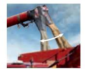
The pivot spout option is operated with the multifunction handle and directs the grain stream into the grain cart, filling it without spillage to maximum level.
