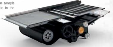
But it's not just the rotor that makes the Axial-Flow® different. The Cross Flow cleaning system which follows the separation process, uses chevron-shaped fins to create a uniform vortex along its axis to generate high volumes of air throughput. Unlike conventional systems, there are no air pockets created – distribution is consistent across the underside of the sieves – and fan speed is fully adjustable to cater for finer-seed crops.
