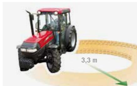
Radio de giro de 3,34 m (Quantum 65V-85V/N/F) y 3,44 m (Quantum 95 and 105 V/N/N/F).
