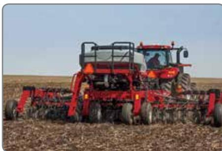
**Precision Disk™ 500 or 500T disk drills** will seed into a variety of tillage systems, from full till to no-till with few adjustments. These drills cut through the heaviest residue with 18-inch disks set at a 7-degree angle to easily slice open a high-quality seed trench.
