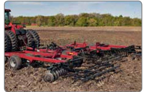
Ideal for primary tillage, seedbed preparation or chemical incorporation, **True-Tandem™ disk harrows** provide straight, easy pulling, maximum pass coverage and level output — especially on rolling ground. The result is properly sized residue, thoroughly mixed soil and effectively incorporated chemicals.
