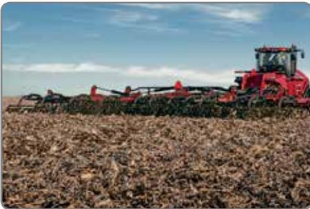
**True-Tandem™ 330 Turbo and 335 VT vertical tillage equipment** incorporate residue and maximize nutrient availability using an exclusive blade design which is perfect for the pre-set gang angle. The low-concavity wavy, fluted blades size Bt corn stalks and break up corn root balls by better cutting and penetrating, and putting sized residue in contact with the soil.
