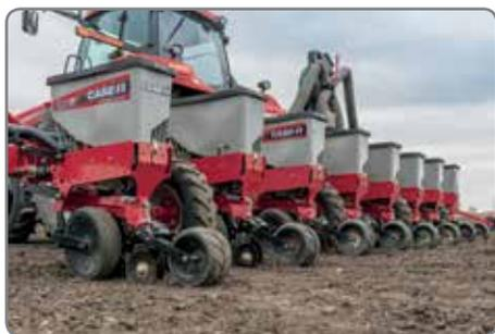
Named the No-Till Product of the Year two years in a row, the **Early Riser® planter** features leading edge, offset disk openers to slice through residue and maintain uniform seed placement in mulch-till or no-till. Case IH field trials show growers can expect 3-4 days earlier emergence and 6-10 percent net effective stand improvement compared to conventional planters<sup>1</sup>.
