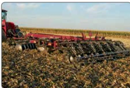
With its Earth Metal 24- or 26-inch blade, the **Ecolo-Tiger® 875 disk ripper** reduces residue size, while the Tiger points fracture soil compaction under the hardpan. It's the most aggressive residue-sizing and mixing option on the market.
