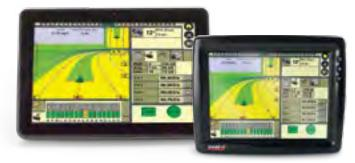
The XCN-2050 and FM-1000 displays in the tractor communicate guidance information to the TrueTracker system, providing repeatable accuracy to improve seedbed and nutrient placement, helping to enhance crop stands and yields.
