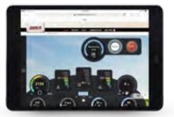
Cellular RTK Guidance (NTRIP) (AFS Connect) Cellular RTK network provides self-propelled windrowers with sub-inch accuracy to minimize overlaps.
