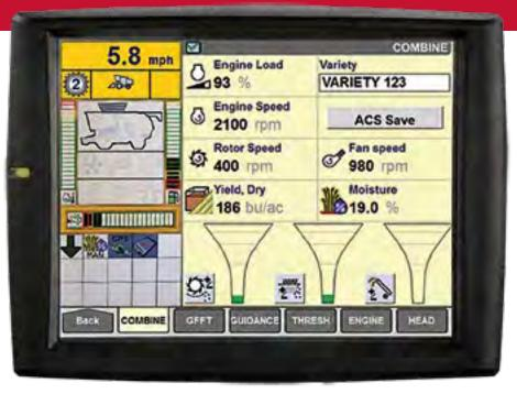
The AFS Pro 700 display runs six screens on a single monitor that allow you to control key machine functions.
