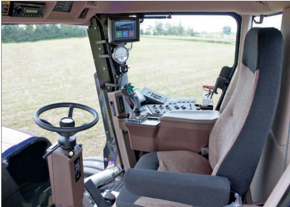
*The deluxe Guardian cab provides outstanding visibility, a high-back air-ride seat of a smooth comfortable ride, and convenient armrest console and joystick control handle for fingertip control.*
