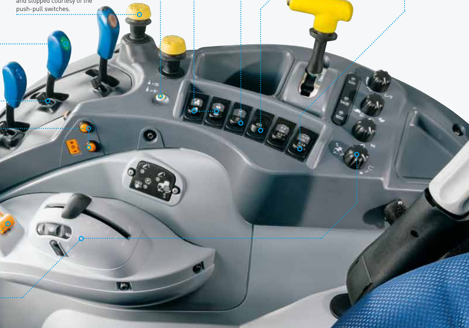
Use Engine Speed Management to pre-set two engine speeds.
