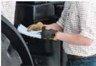
Engine oil check and fill points are easy to reach, with no need to lift the hood. This makes routine checks faster and servicing simpler. You will also still be able to enjoy the long 600 hour service intervals that you've come to expect of New Holland.
