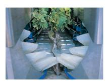
2 chain of baskets on each side receive the falling berries from shaking system. Ground losses are minimal because of the perfect sealing.Full respect and no damage to the stock.
