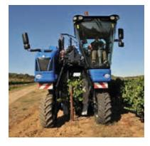
NH grape harvesters are straddle-type: 2 wheels on each side of the row. It does not damages the canopy, but interspacing size must be fit for access to the rows.
