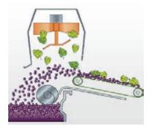
Berries are unloaded from the Noria in two tanks, the crop is spread onto belt conveyors: in the meanwhile, suction fan cleans harvest from leaves and other unwanted material. Fan speed is adjustable for fine tuning of cleanliness expected.
