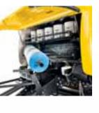
Integrated prop to support a roll of net when changing it from ground level.
