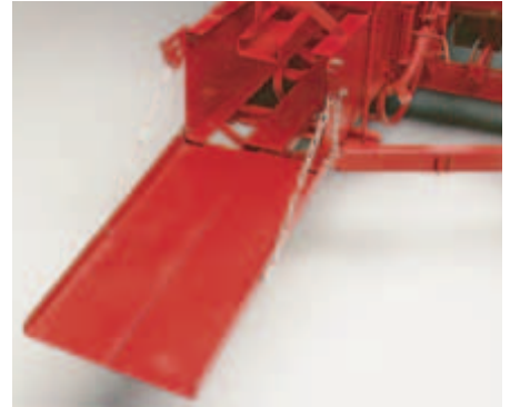
Triple-purpose chute supports bales as they leave the chamber; can be set to roll bales to the left, away from the next windrow. (Also becomes the base for bale-loading chute.)
