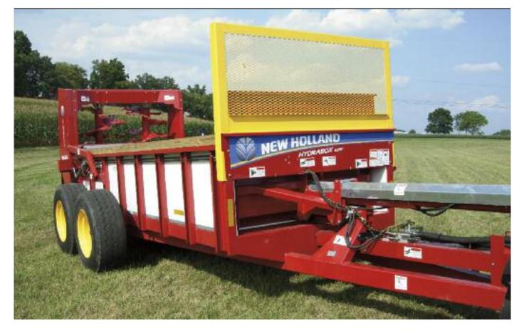
HydraBox<sup>™</sup> hydraulic-push box spreaders from New Holland are built for simplicity, easy maintenance and years of productive performance. These spreaders uniformly spread solid and semi-solid manure, poultry litter, bedding material, soil amendments, mulch and compost.
