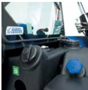
Access to the 140 litre fuel tank is via a wide opening filler, allowing in-field refuelling with cans if ever necessary. With a capacity of 27 litres, the AdBlue tank is large enough to last for at least 5 fuel tank fills.
