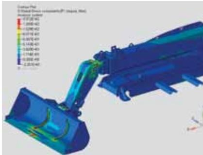
Based around twin U-shaped 10mm to 12mm thick sections, the completely new boom is immensely strong, with heavy duty pivot pins for optimum durability. New wear pads adjust quickly using a simple screw and lock nut design, without the need for special tools.
