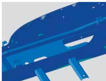
The one-piece H shape ladder chassis is made from 25mm thick, high tensile steel that is fully robot welded to ensure exceptional torsional rigidity. The boom support is exceptionally strong, its mass helping to counterbalance heavy loads.
