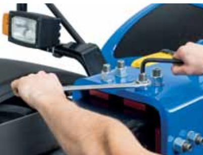
The once time consuming job of adjusting the telescopic boom pads has also been simplified, a simple nut screw and lock nut system making adjustment quick and easy.
