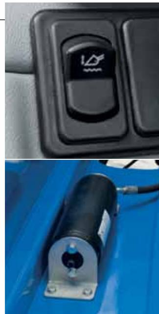
Boom suspension can be specified. The system is activated by the operator and is designed to help reduce shock loads when working over difficult terrain. The system automatically deactivates when the boom exceeds a 35 degree lift angle.
