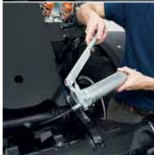
On Standard models, there are just nine daily grease points, Elite models having three extra on the high tip angle carriage. Every grease point is designed to be easy to access with remote greasing for those that would otherwise be difficult to reach.
