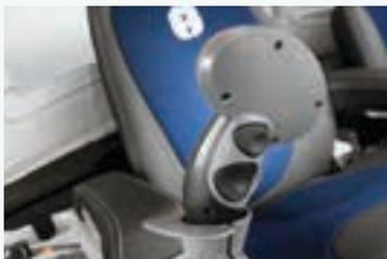
Shift button and ground speed unlock (behind).
