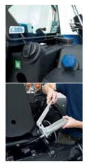
Access to the 140 litre fuel tank is via a wide opening filler, allowing in-field refuelling with cans if ever necessary. With a capacity of 27 litres, the AdBlue tank is large enough to last for at least 5 fuel tank fills.
