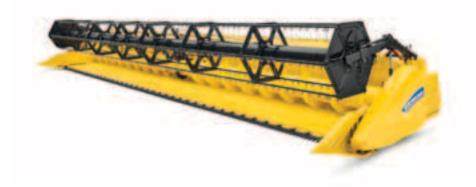
Varifeed™ headers benefit from a full 575mm of knife adjustment for guaranteed harvesting efficiency and correct feeding. What's more, you can adjust the knife position right from the comfort of the cab.
