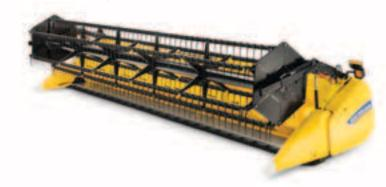
Maintain uniform stubble height in uneven fields. How? The header flexes up to 10cm to follow the ground contours perfectly thanks to an exclusive and patented rubber spring floatation system.
