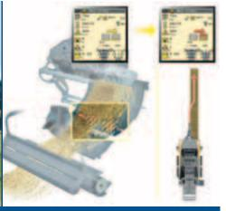
Uniform bales. Every time. SmartFill™ technology uses a network of sensors to ensure uniform flake formation, and informs the drivers of where to drive to maintain this.
