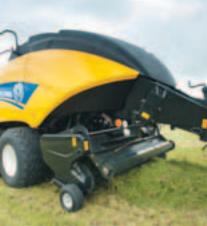
MaxiSweep™ pick-up Smooth crop flow is guaranteed courtesy of the new roller wind guard and feed assist rollers. Crop is more efficiently transferred into the chamber by the contrarotating under and overshot augers.
