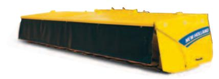
Delivering one-pass, high speed harvesting, the six metre Marangon for New Holland header scythes through whole crop and grass thanks to its 14 cutting discs which guarantee a super fine cut.
