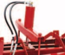
Maintaining consistency bale density Hydroformatic density control maintains bale density independently of crop moisture content.
