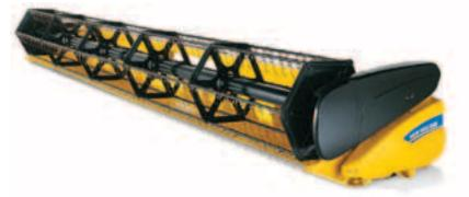
For smooth crop guidance to the knife and to the feed auger, the High Capacity header has a large reel diameter and easy reel adjustments.
