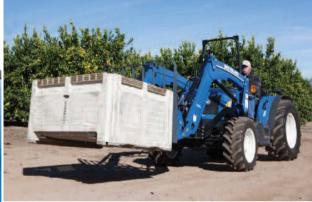
Note: The TD4040F tractor pictured above has a mid-mounted ROPS. On this particular configuration, the mid-mounted ROPS may help to protect an operator from a large object falling down the loader arms. However, on tractors with a rear-mounted ROPS operating a with a loader, a FOPS is recommended to protect the operator from large objects falling down the loader arms.
