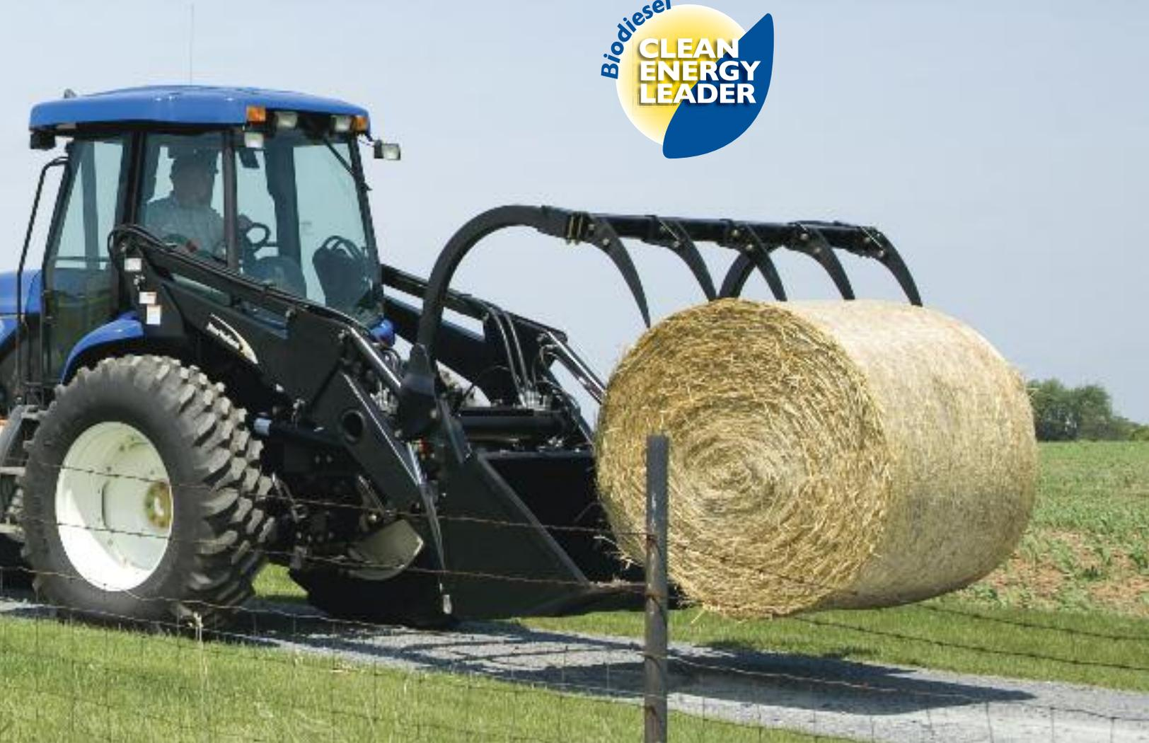
ward and you move forward. The further you push, the faster you go. Pull it back and the tractor slows gradually and shifts into neutral, then reverse. No clutch needed. It's the best shuttle shifting you'll find, which makes the TV6070 ideal for loader work.
