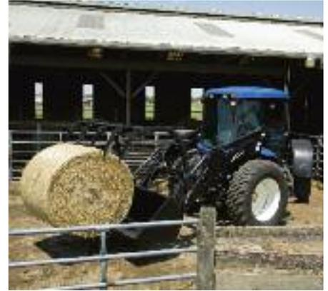
*Articulated steering lets you make sharp turns and maneuver in tight areas a typical tractor can't. If one end of the tractor fits, the other end will, too.*
