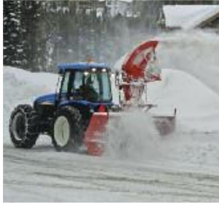
*True four-wheel drive with four equal-size tires provides superior traction in wet, icy or muddy conditions.*
