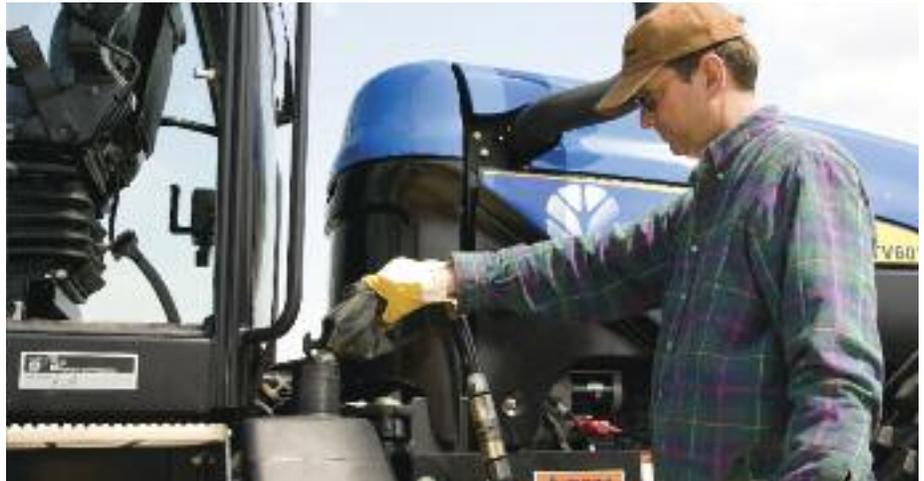
*The high-capacity 55-gallon (total capacity) fuel tanks are located in front of the cab steps and can be reached conveniently from the ground and filled from either side.*
