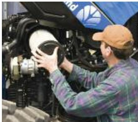
*The engine air filter is accessible from ground level. Easy, spin-off wing nuts make cleaning or replacement a breeze.*
