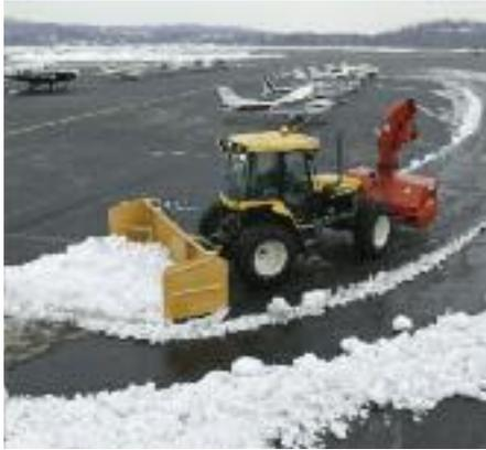
*You get double-duty with the Bidirectional™ tractor. A PTO, three-point hitch, and drawbar at each end let you push and pull implements at the same time, doubling your productivity.*
