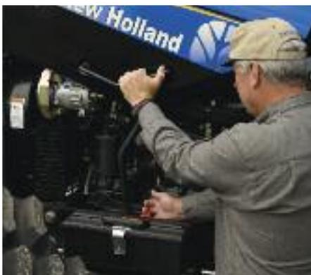
*Pull this lever and the entire hood flips up for complete engine access.*
