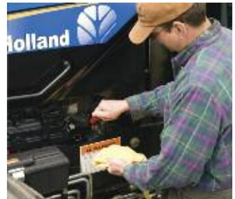
*The oil dipstick and fill port can be reached without lifting the hood.*
