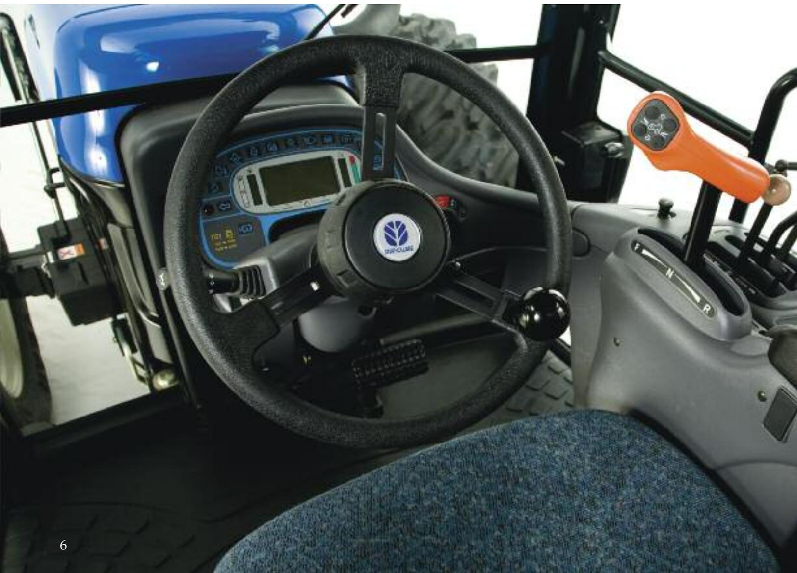
and remain that way regardless of which direction you're facing. Whether the console is facing the cab end or the engine end, it can be offset 15 degrees as a single unit for added comfort when looking back. And, since the cab has two doors, you can enter or exit the cab from either side, depending on the position of the Turnabout console.
