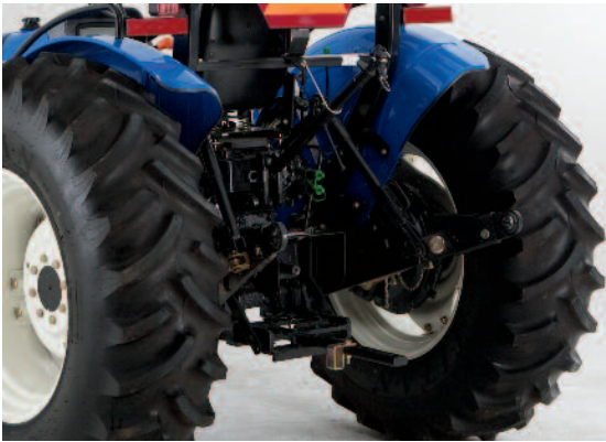
Implement hookup is a snap since WORKMASTER tractors come standard with flexible link ends, telescoping stabilizers and a swinging drawbar.
