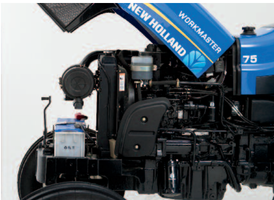
Flip-up hood provides fast, complete access to service areas with no panels or grills to remove.
