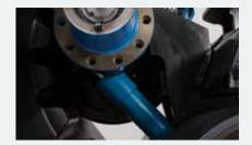
6 Integrated accumulator/ tensioner automatically adjusts belts for proper tension.
