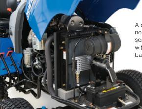
A one-piece hood with no side panels makes serviceability simple with easy access to the battery and air filter.
