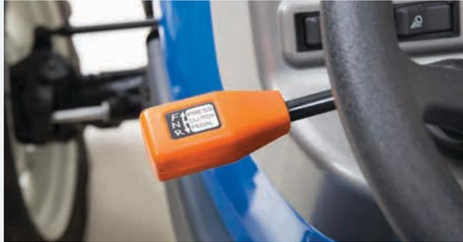
**Convenient 8 x 8 synchronized shuttle transmission**
