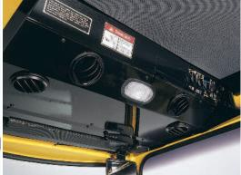
Adjust the direction and flow from the overhead air conditioning and heater vents for maximum comfort.
