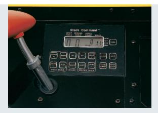
The Stack Command<sup>™</sup> control system provides up to 35 pre-programmed stack patterns as well as room for 20 custom patterns that you can program.
