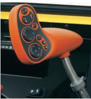
All machine functions are conveniently located on one multi-function handle.
