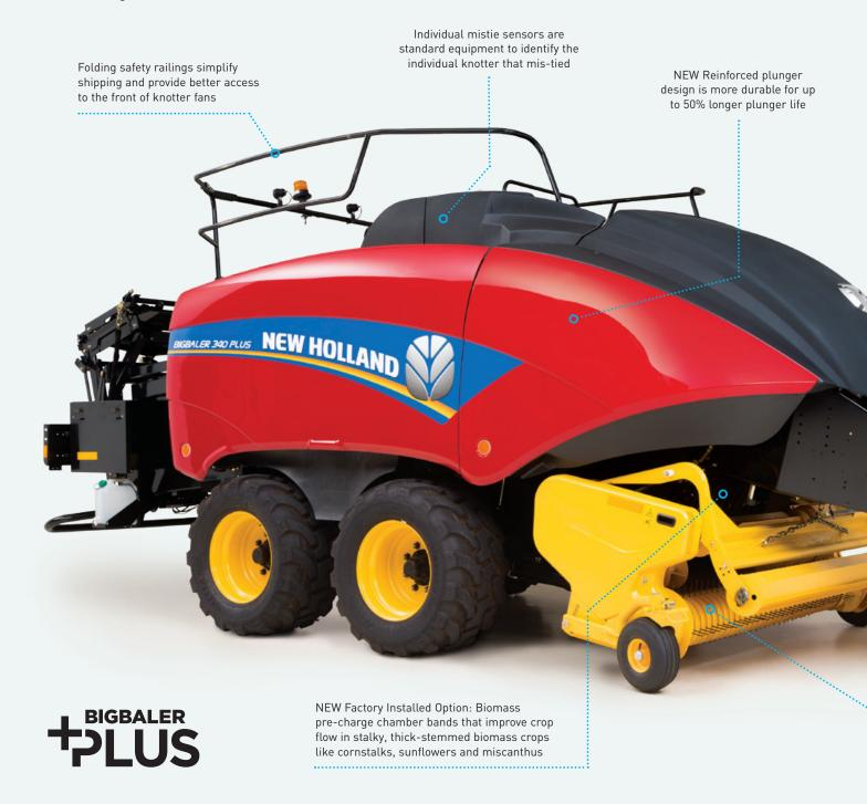
The wide baler body includes a larger platform to allow for easier cleaning of the sides of baler
