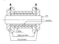
Oil applied to rollers only cannot reach pin-bushing joints, and therefore, cannot retard chain elongation due to wear. The lengthening of chains in service results from wear on pin and bushing surfaces, not rollers. When lubricating multiple strand chain, it is important that lubricant be directed to each row of chain linkplates. In conveyor applications, oil should be directed between the rollers and bushings as well as between the chain linkplates.
