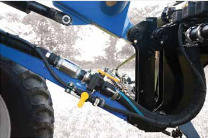
The convenient Guardian™ Quick-Attach option allows you to separate the Injection Toolbar from the chassis quickly and easily.
