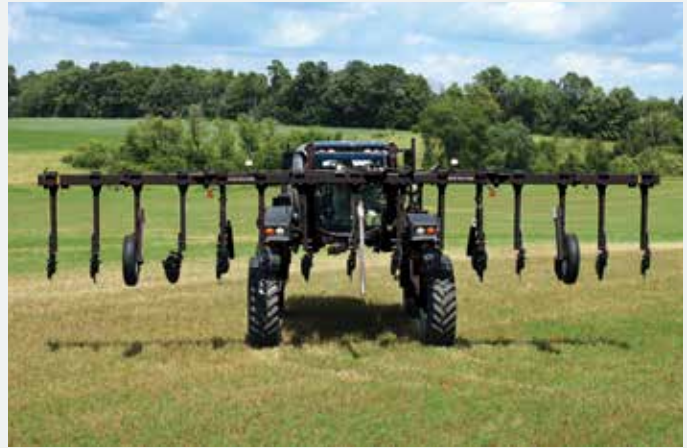
High lift clearance helps the coulters clear crops and obstacles at the headlands, minimizing the potential for damaging corn stalks.
