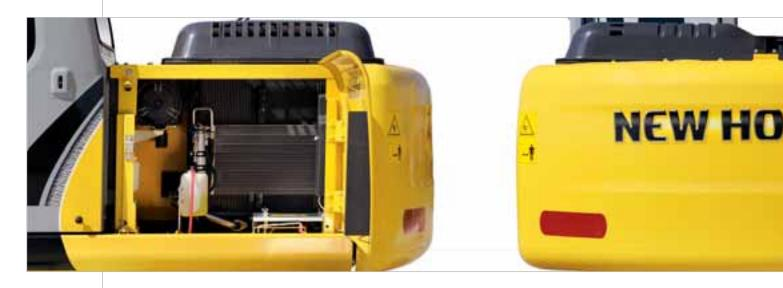
L he simplified byout of all vial components of the New Holland E135B under both the right and the left side panels makes maintenance much easier, less time consuming and less costly, and provides much better access for servicing. There is plenty of room in all compartments and most components are positioned in such a way to enable easy access from ground level. An elegant and modern design added to state-of-the-art technology.
