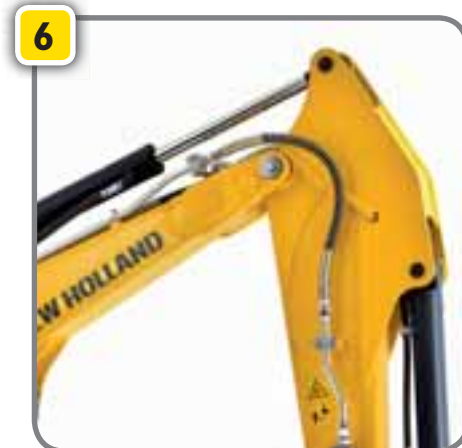
Reinforced boom/arm connection
