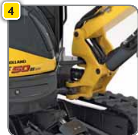
Molded boom swing articulation + No exposed hoses = long life
