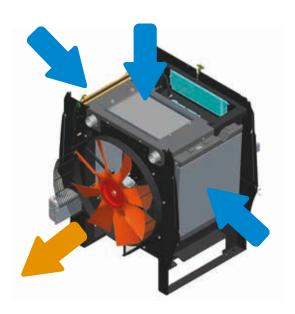
In dusty environments like sand pits or quarries the cleaning of the radiators can be very time consuming: that is not the case with the cooling cube.
