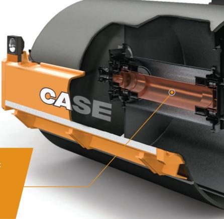
The centrifugal force is generated by an internal eccentric shaft and a rotating mass: depending on the direction of rotation, the rotating mass is in phase with the eccentric shaft for a maximum centrifugal force or in the opposite position, for a minimum centrifugal force.
