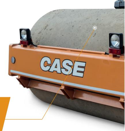
The centrifugal force is generated by an internal eccentric shaft and a rotating mass: depending on the direction of rotation, the rotating mass is in phase with the eccentric shaft for a maximum centrifugal force or in the opposite position, for a minimum centrifugal force.
