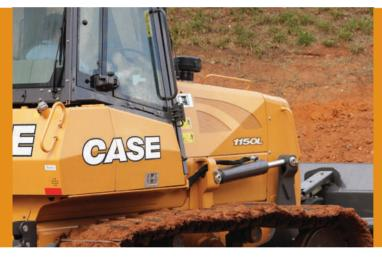
**ADJUSTABLE BLADE PITCH** The low-effort blade hydraulics feature powerful cylinders able to move the blade with ease and control. The mechanical pitch blade can be set between 50 to 60 degrees to suit every dozing application and ground condition.
