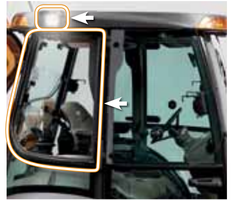
New rear-quarter windows and side lighting
