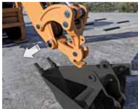
Factory supplied hydraulic and mechanical quick coupler options.
