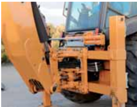
Rapid hydraulic side shift (in option), in under 5 seconds.
