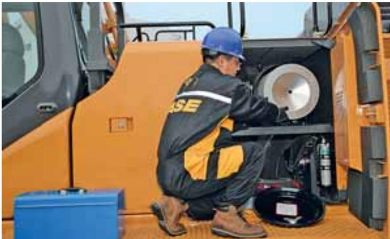
The CX800B uses Extended Maintenance System (EMS) bushings on all pins except for the attachment linkage. EMS bushings allow 1,000 hour greasing intervals, with 250 hour intervals on the attachment pins. Anti-friction shims further reduce wear on the boom foot and head linkage, cutting noise and operating cost for the customer.
