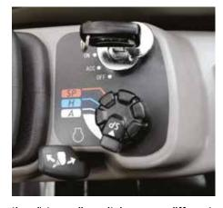
Operators can store up to 10 auxiliary hydraulic flow settings (and pressures as optional) to easily switch among different attachments with no need of any mechanical adjustment.
