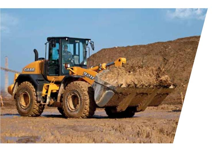
With L5 tyres, needed for work in very abrasive environments, we recommend heavy-duty axles. Solid tires can be retrofitted
