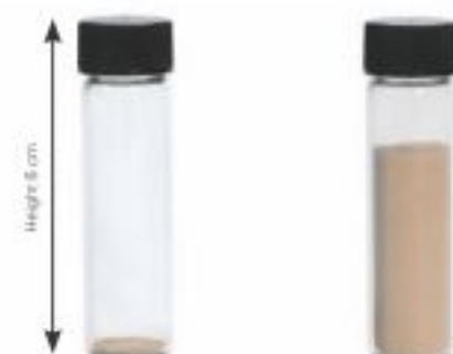
Contamination levels of Different ISO 4606 Codes Vary Dramatically*
