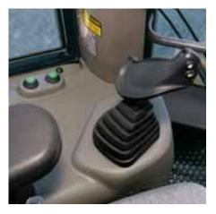
There's absolutely no need to brake or lift the blade to lighten the load when turning—no wonder we call it "Power Steer." This means you'll make fewer passes to move material for greater productivity. You'll find these dozers are much more productive than competitive machines using clutch and brake steer systems. And the Power Steer feature makes the dozer easy to run, improving productivity, reducing operator fatigue, and lowering operating cost per cubic yard.
