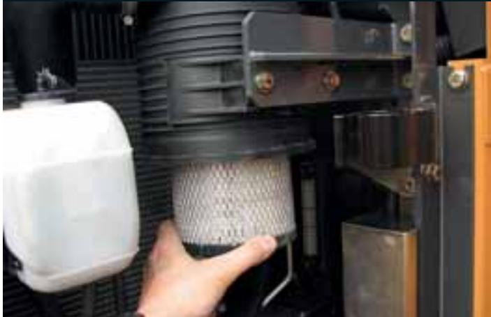
Remote-mounted filters in the hydraulic pump area offer ground level servicing, with green drain cocks for engine oil preventing spillage on sensitive ground. The fuel tanks are enlarged, which in combination with reduced fuel consumption results in longer running between refuelling stops, cutting downtime and boosting productivity. EMS bushing on the boom and dipper offer up to 1,000 greasing intervals, further reducing service times and lowering operating costs.
