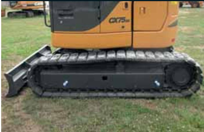
Case undercarriage design promises long component life and low operating costs. Case excavators have heat treated drive sprockets for extended use. Robust track guides and improved track links, with new M-shaped seals and increased pin hardness, further boost durability and reliability. The track rollers have a revised profile for lower wear, and the O-ring design prevents the ingress of abrasive material, further extending longevity.
