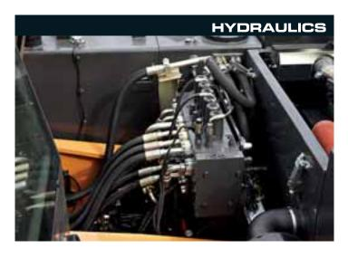
The WX240 features a well laid out, easy to maintain hydraulic control valve. The Case Digipower hydraulic control system monitors the main pumps and regulates engine power to meet the needs of the operator. All WX machines offer a range of selectable power levels, or working modes, for specific digging and lifting tasks. These include a levelling mode for fine grading work. PowerBoost is standard in the lifting modes and works for 8 seconds in all other modes according to operator demand.
