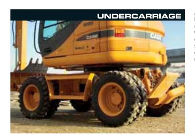
A two gear range transmission offers a maximum travel speed between job sites of 33 km/h. Maximum drawbar pull in low range is 62 kN. The WX95 Series 2 can be specified with two wheel steering or four wheel steering, and a choice of single or double wheels. In four wheel steering the machine offers a crab steering mode to allow diagonal movement away from a wall or obstruction, protecting the upperstructure and reducing the risk of impact on site.
