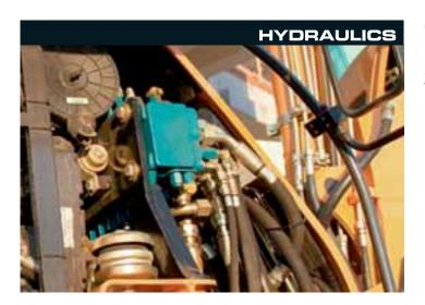
Case has been a manufacturer of class-leading excavators for many years and the WX95 Series 2 builds on that success. The hydraulic system has on-board computer and engine speed sensor control to maximise hydraulic flow and pressure to meet the operator's needs. A swing pressure control offers the driver outstanding controllability, while the flow pump saving circuit minimises oil return to ensure smooth flowing movement of the boom and dipper arm.
