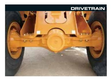
The 521E wheel loaders use a torque sensing autoshift transmission with four forward gears and three reverse ratios. The operator can choose to use the transmission in manual or full auto modes. Top forward speed is 39 km/h.
