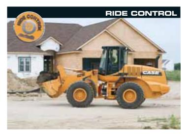
Material retention and operator comfort can be further improved with the addition of optional Ride Control, a system that allows the lift arms to float when the machine is moving. This prevents bounce in the cab and at the wheels. Ride Control permits higher travel speeds during load and carry operations, reducing fatigue for the operator and increasing productivity.
