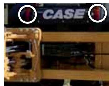
Rear road lights can be fitted on the stabilizer legs while traveling and on the cab when digging, providing maximum visibility and protection
