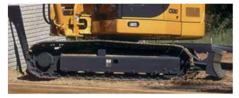
LC type undercarriage providing excellent stability (as a result of its length) and loading capacity comparable to machines of standard dimensions.
