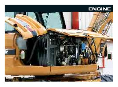
Electronically-controlled turbo charged diesel engine meets Tier III emissions regulations. In tests the 112 hp (84 kW) engine offers increased productivity with up to 12% lower fuel consumption. Engine and hydraulic pump monitoring and control system offers multifunction use with high output, increasing productivity and tonne/litre output for the customer.
