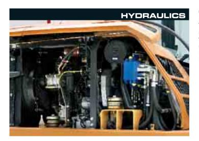
Case has been a manufacturer of class-leading excavators for many years and the WX125 Series 2 builds on that success. The hydraulic system has on-board computer and engine speed sensor control to maximise hydraulic flow and pressure to meet the operator's needs. A swing pressure control offers the driver outstanding controllability, while the flow pump saving circuit minimises oil return to ensure smooth flowing movement of the boom and dipper arm.
