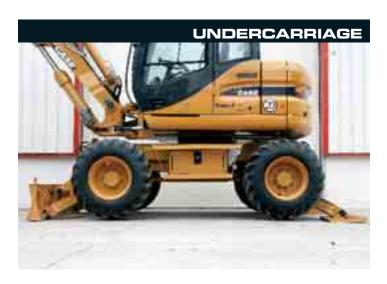
A two gear range transmission offers a maximum travel speed between job sites of 33 km/h. Maximum drawbar pull in low range is 79 kN. The WX125 Series 2 can be specified with two wheel steering or four wheel steering, and a choice of single or double wheels. In four wheel steering the machine offers a crab steering mode to allow diagonal movement away from a wall or obstruction, protecting the upperstructure and reducing the risk of impact on site.
