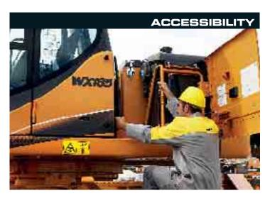
Even with the reduced tail radius of the Case WX, the machine retains the Case access catwalk behind the cab, offering the service engineer excellent access to the regular service and maintenance points and providing a safe working area. A lift up engine canopy provides a clear view to the top of the engine, the hydraulic valves and the cooling pack.
