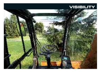
Large glass area with two-piece full height front windscreen offers unparalleled visibility all around the machine. The operator has a clear view to the work area when digging and loading, and to the road ahead when travelling the machine between job sites. A low engine canopy to the rear of the machine provides a clear view behind the excavator when manoeuvring on confined sites.
