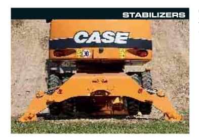
Customers can choose between a stabilisers, blade or a combination of the two, thanks to the modular design of the Case WX chassis. The stabilisers and dozer blade are independently controlled, to allow for levelling on rough ground.
