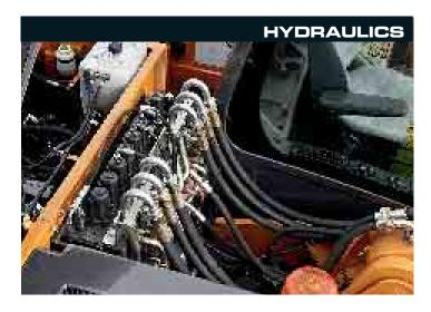
Clean, easy to maintain hydraulic valve layout. The Case Digipower hydraulic control system monitors the main pumps and regulates engine power to meet the needs of the operator. The WX machines offer a range of selectable power levels, for specific digging and lifting tasks, including a levelling mode for fine grading work. PowerBoost is standard in the lifting modes and works for 8 seconds in all other modes on request.
