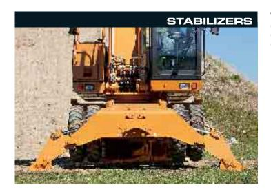
With the modular design of the Case WX chassis, customers can choose between stabilisers, a dozer blade or a combination of the two. The stabilisers and dozer blade are independently controlled, to allow for machine levelling on rough ground.
