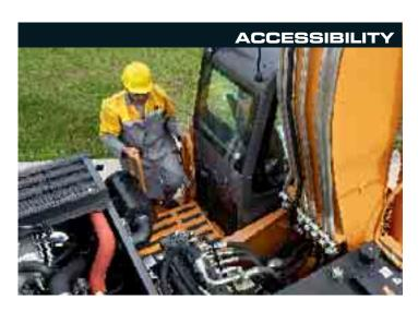
The machine retains the Case access catwalk behind the cab. The service engineer has unparalleled access to all regular service and maintenance points and a safe area in which to work. The top of the engine, the hydraulic valves and the cooling pack are easily accessible through the large lift up canopy.
