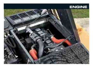
The WX240 uses a six cylinder Case engine for maximum torque and smooth power. This EU Tier III compliant engine is turbocharged and intercooled for optimised clean combustion and high power output. The engine has been designed for maximum reliability and durability, with an auto warm-up feature ensuring long service life and reduced downtime.
